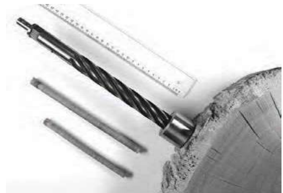
This image shows a drill that’s used by dendrochronologists to take samples from trees. (Courtesy of Hannes Grobe/AWI, CC-BY-SA-2.5, Wikimedia Commons .)
